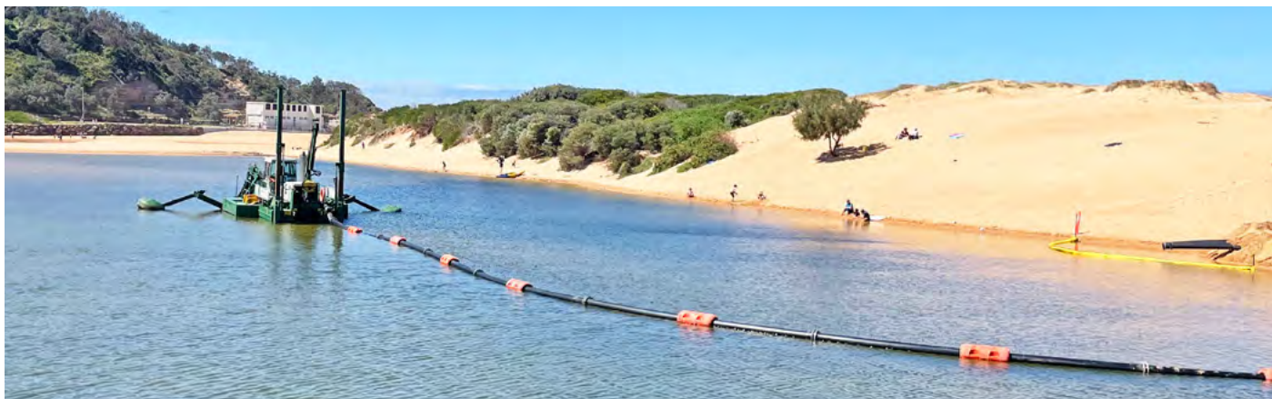
Protecting the local community from flooding in a smart way Watermaster dredgers pumped the accumulated sand directly to the shore in one go
