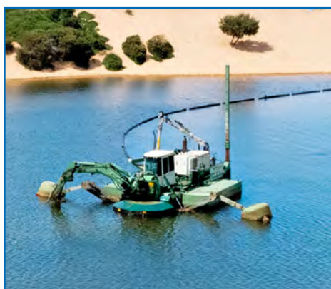
Watermasters suction dredge the accumulated sand directly to the shore
