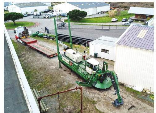
The ease of changing a site - Watermaster transports as a complete unit, it unloads from the trailer and walks into the water by itself
