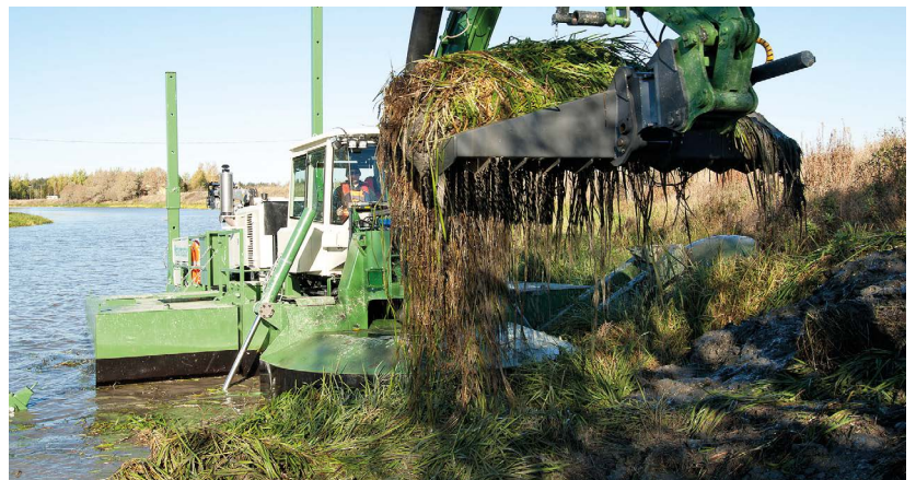
Removing excessive vegetation - with the rake tool Watermaster removes floating and rooted aquatic vegetation (picture from Finland)
