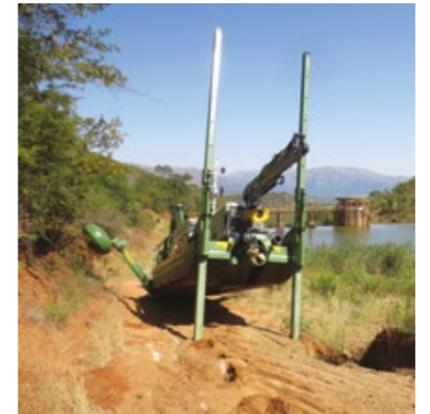
No cranes or tugboats required - the amphibious Watermaster moves independently on land and in water.
