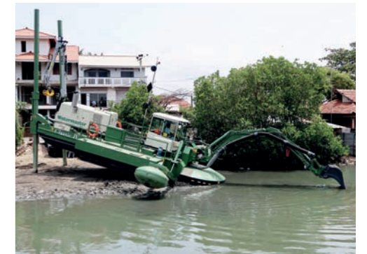
Watermaster is fully amphibious - it is a vessel certified for work both in water and on land.
